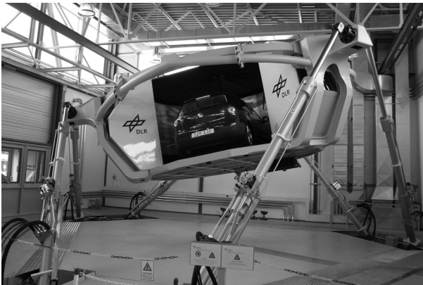
Fig. 1. Dynamic driving simulator at the German Aerospace Center
