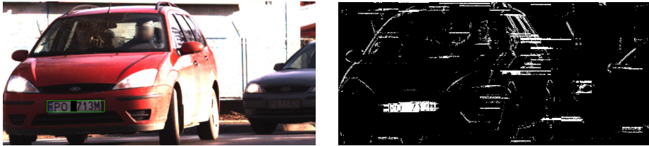
Fig. 1. The output (right) of the best-of-run individual of one of the GP-IFS runs, when applied to the input image shown in left inset. Pixel brightness reflects individual's confidence in the presence of plate. The plate has been obfuscated due to privacy concerns.
