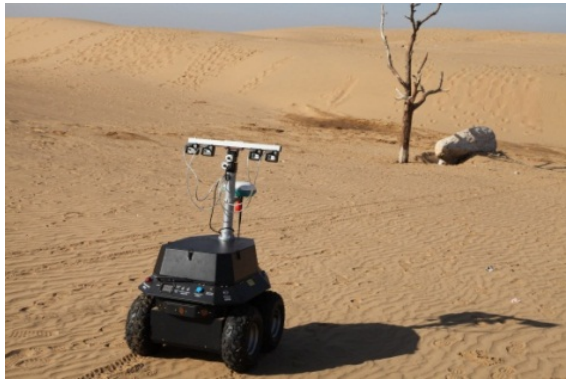
Fig. 3. Field test of visual tracking for target approach on a model rover
