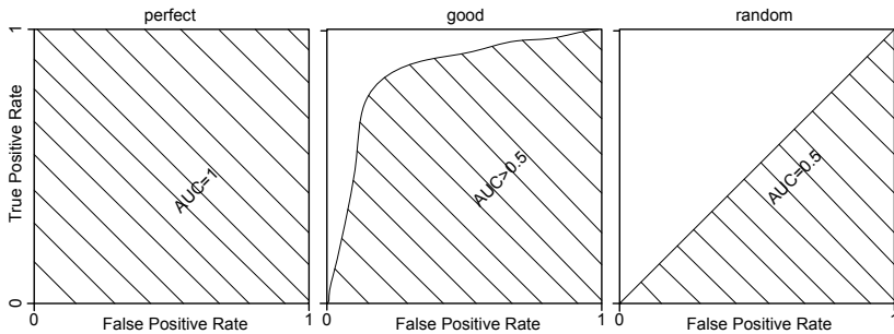
Fig. 1. ROC curves for classifiers of different quality. Leftmost is the case of perfect classification, the rightmost is random guessing.
