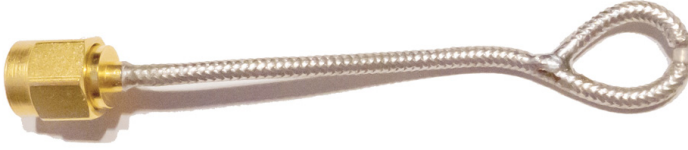
Fig. 5. Shielded magnetic field probe, before wrapping in an insulator to allow safe probing of any area of the device under test
