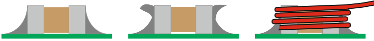
Fig. 14. Winding the pickup coil around an arbitrary decoupling capacitor is achieved by adding a form with solder. In addition the choice to connect one side of the coil to the ground of the circuit simplifies connection of the oscilloscope in some situations.
