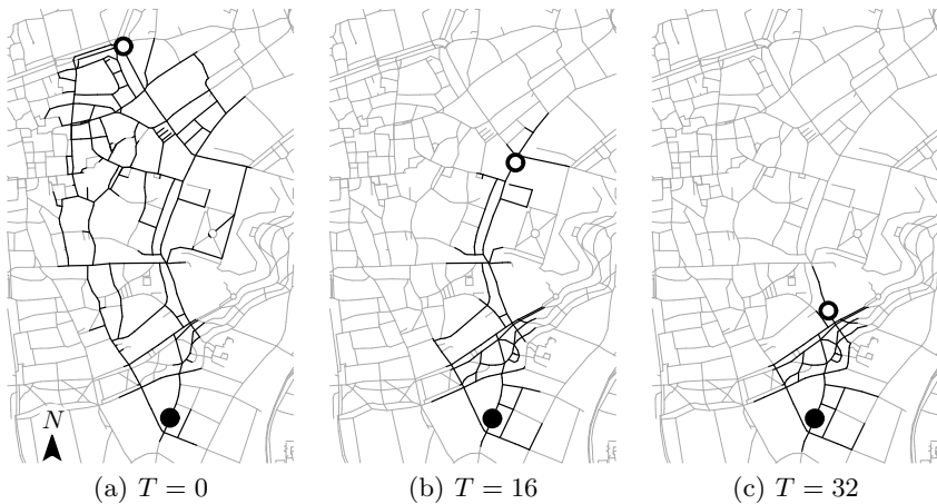
Fig. 2. Several edge selections while a user travels a shortest path to a destination. The value T indicates the number of road segments traveled. Current user location is marked with \circ , destination is marked with \bullet .
