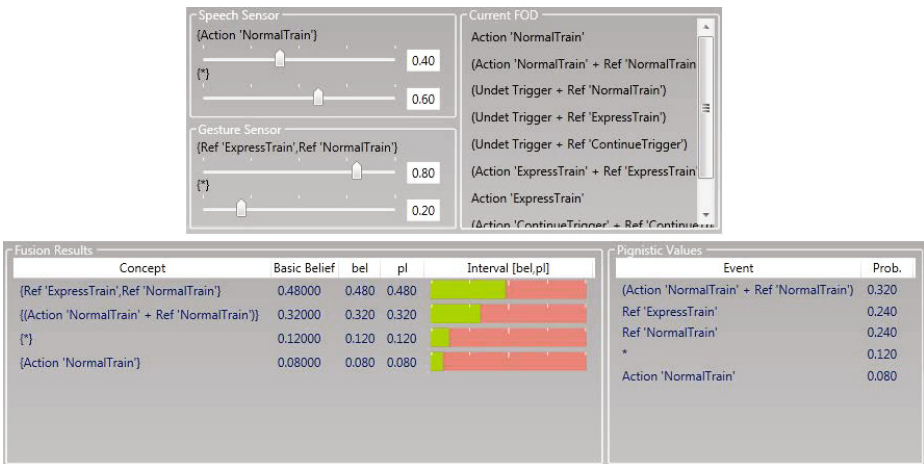
Fig. 4. Screenshot of the fusion system, where low confidence and ambiguous inputs (top left) are combined resulting in the highest probability for the correct event (lower right)
