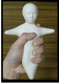
Fig. 1. Elfoid: cellular-phone-type teleoperated android
