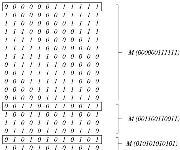
Fig. 2. A solution to Reconstruction(H, V, C) when the horizontal projections have constant value 6, and the vertical projections 9. The submatrices M(u) obtained by row wise arranging the elements of three necklaces are highlighted. Note that M((0011)^3) and M((01)^6) are the only two possible necklaces of length 12 and density 6 having 4 and 2 rows, respectively.
