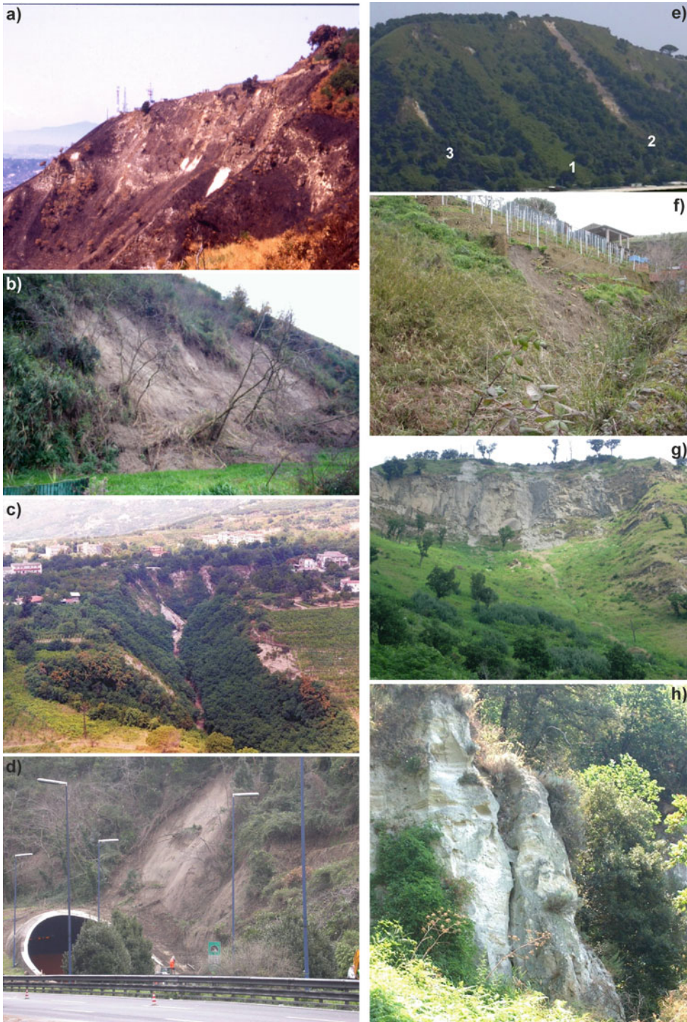
Fig. 5 Recent slope instabilities of the Neapolitan-Phlegraean area. a Post-fire shallow slides along the southern slope of the Camaldoli Hill (Naples, summer 1996); b Typical small-scale slide along the inner slope of the Agnano Plain (Naples, January 1997); c Cluster of slides at the border between Naples and Quarto (January 1997); d Translational slide that invaded the Naples bypass (Tangenziale) (Pozzuoli, March 4, 2005); e different generations of translational slides along the western
