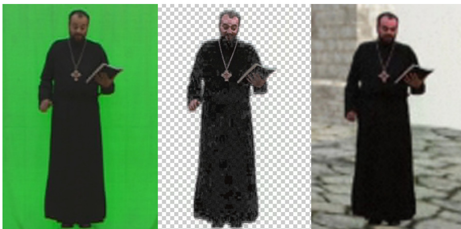
Fig. 4. Keying the footage: virtual guide against the green screen (left); virtual guide keyed out with alpha channel (middle); virtual guide superimposed on the virtual model (right)
