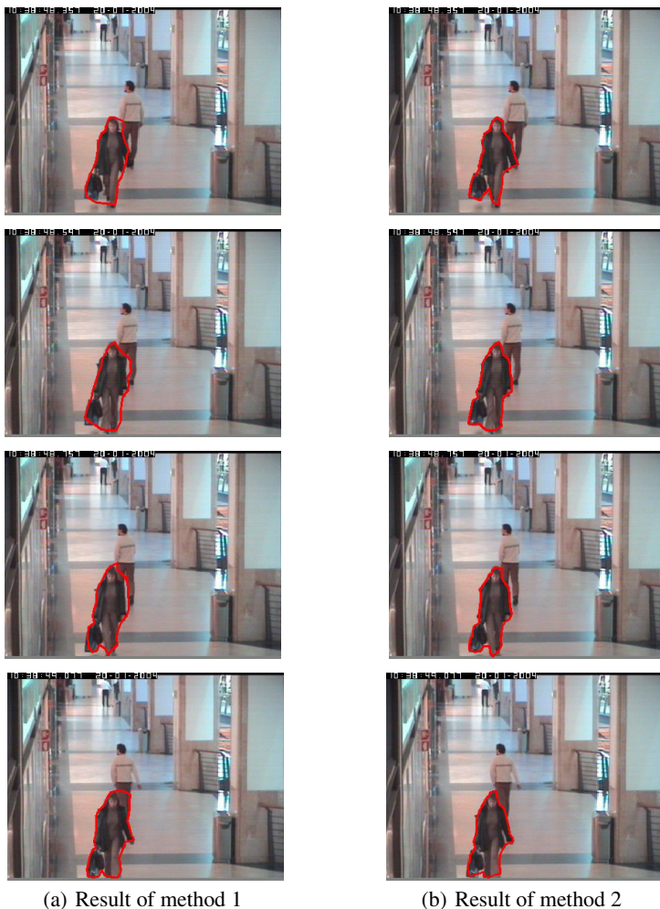
Fig. 5. Pedestrian sequence with occlusion. The red closed curve indicates the contour. From top to bottom are the frames 254, 260, 265 and 272. Column (a) is the result of method 1, (b) is the result of method 2 (our method).
