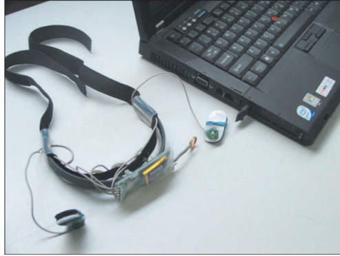
Fig. 1. The prototype of mobile EEG belt. Three recording electrodes (Fp1, Fp2 and Fpz) are placed on the forehead complying with the international 10-20 system, with the reference and ground electrodes on the ear lobes.
