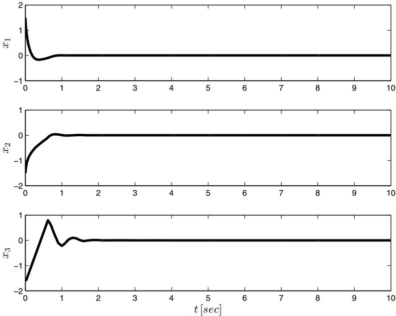
**Fig. 14.5** The system's state vector  $x$  converges to zero
