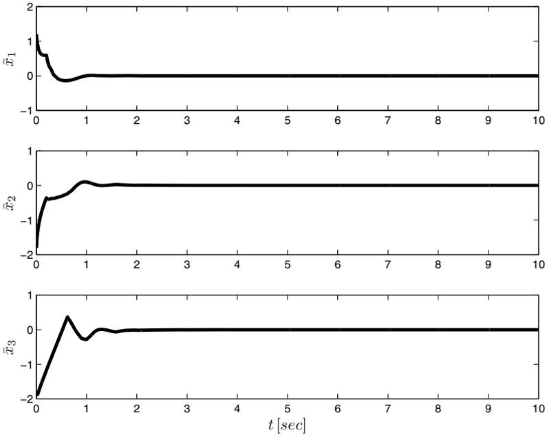
**Fig. 14.4** On  $s(\bar{x}) = 0$  the observer's state vector  $\bar{x}$  converges to zero
