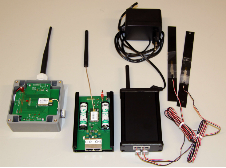
Fig. 2. Wireless strain measurement devices (SINK and nodes) and attached strain gauges
