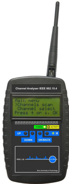
Fig. 4. Photography of developed channel analyzer
