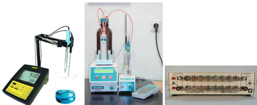
Fig. 9.4 Some examples of modern measuring devices. Left ordinary pH meter with a glass pH electrode and a reference electrode; middle titrator with electrodes to control the titration process; right multichannel EMF measuring station: the potentials of up to 16 ISEs can be measured simultaneously
