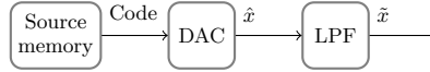
Fig. 2. (Arbitrary waveform generator) the code specifies the levels of discrete signal \hat{x} , which the low-pass filter smooths to create \tilde{x} (NOTE: \hat{x} has discrete levels but is continuous in time)
