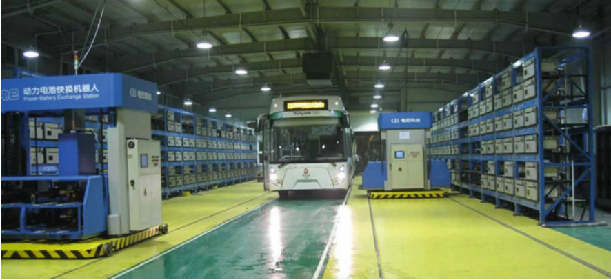
Fig. 9.9 Workshop for changing batteries at a charging station for buses during the Beijing Olympic Games
