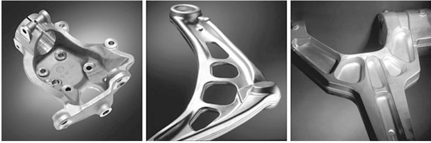
Fig. 3.56 Manufacturing examples of complex closed-die forging parts made of aluminium alloys for use in a chassis— left passenger car swivel bearing, length 250 mm (Source Hirschvogel Umformtechnik GmbH); centre and right passenger car triangle wishbone (ca. 2 kg) of AlMgSi1 and aircraft steering arm nose gear (ca. 180 kg) made of AlZnMgCu 1.5 (Source Otto Fuchs KG)
