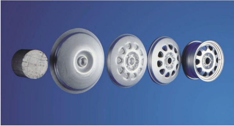
Fig. 3.53 Operating sequence in the manufacture of an alloy wheel rim of AlMgSi1 (Source Otto Fuchs KG)
