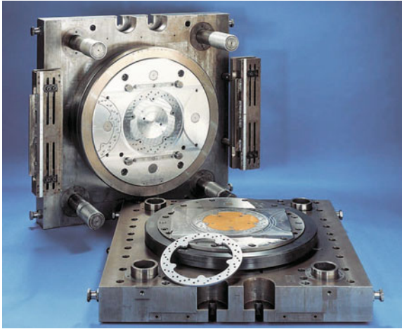
Fig. 5.39 Fine blanking with a blanking and piercing tool ( Source Feintool AG)
