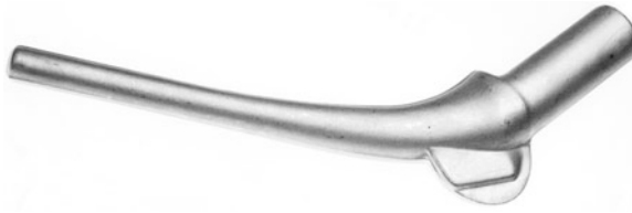
Fig. 3.72 Isothermally forged hip joint prosthesis made of TiAl6V4, length ca. 20 cm (Source Otto Fuchs KG)
