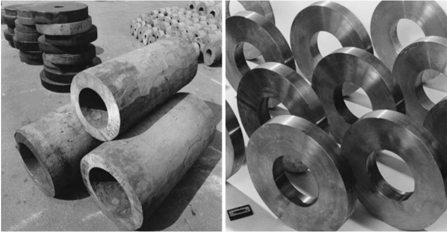
Fig. 3.44 Rings and hollow cylinders manufactured by means of open-die forging (Source Schmidt + Clemens GmbH)
