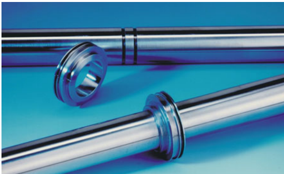
Fig. 3.61 The attachment of a piston on a rack via swaging (Source Gebr. Felss GmbH)
