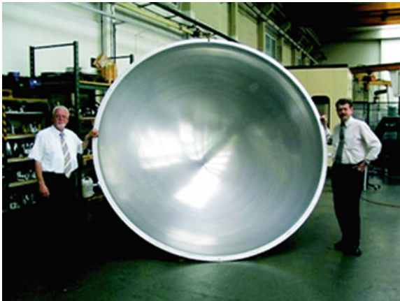
Fig. 4.65 Metal spun fuel tank bottom for a civil carrier rocket (source Leifeld Metal Spinning GmbH)
