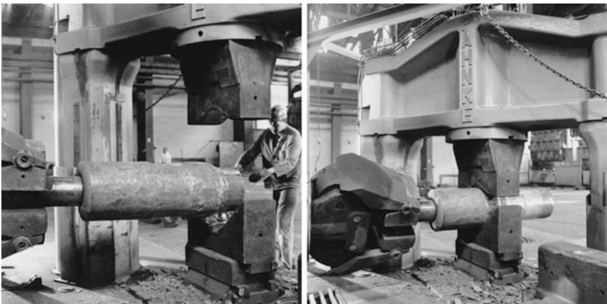
Fig. 3.45 Open-die forging of a hollow cylinder (Source Schmidt + Clemens GmbH)
