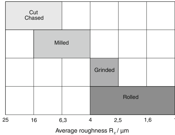
Fig. 3.92 Averaged roughness heights of thread profiles produced in different processes [APEL53]
