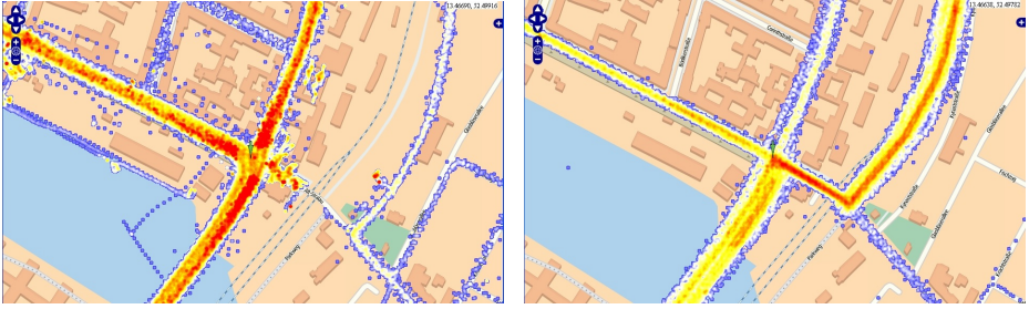
Fig. 9. Density of GPS points. Left (real world data): Standing cars in front of traffic lights produce higher density. Right (synthetic data): Many routes use street which is closed in reality.
