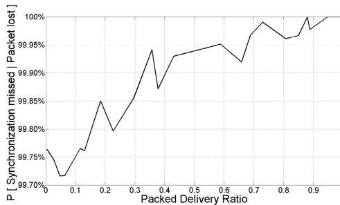
Fig. 2. Probability of a synchronization failure given that the packet is lost
