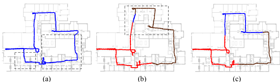
Fig. 7. (a) Trajectory from the single best IPS. Dashed rectangles indicate areas where localization error is larger than 4m^2 . (b) Switching according to FA , and LE_F = 5.33m^2 . (c) Switching according to LA , and LE_L = 2.07m^2 .
