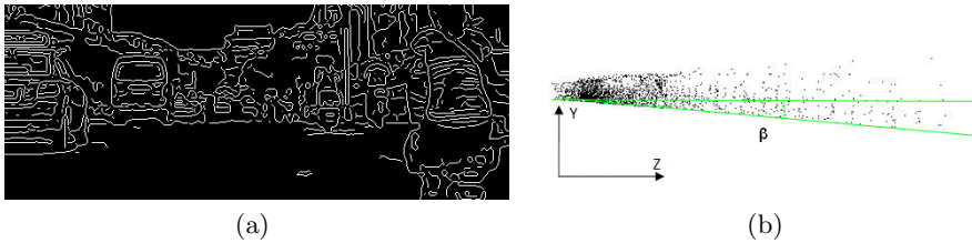
Fig. 4. Edge feature based road fitting. (a) Edge feature of this frame. (b) Feature points projected to YOZ plane, \beta is the angle between road and horizontal.
