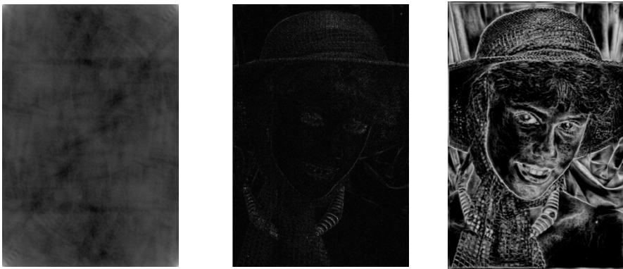
(a) The Reconstruction Image using the Magnitude Map (b) The Reconstruction Image using the Phase Map (c) Phase Congruency Map
