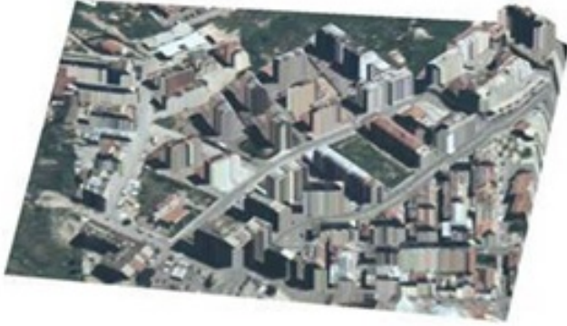
Fig. 2. DEM with overlapping ortho-photos
