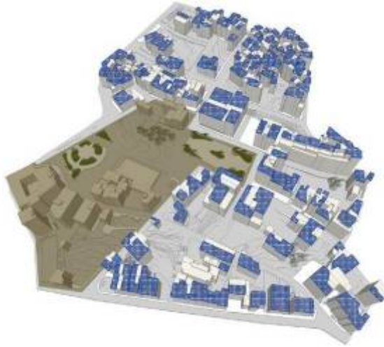
Fig. 7. Rendering of the available areas for the installation of solar systems in the quarter surrounding the city hall
