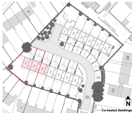
Fig. 1. Site plan highlighting the co-heated plots 6 and 7 as well as the just heated plot 5
