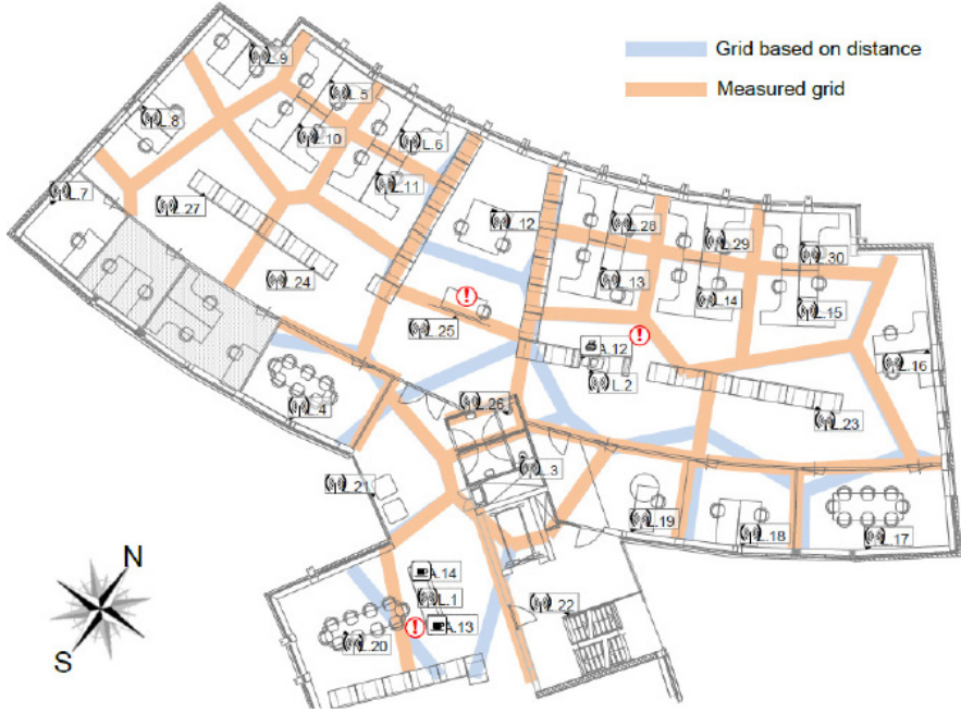
Fig. 8. Floor plan with calculated and measured grid formed by 30 static nodes
