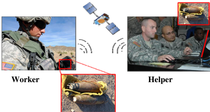
Fig. 1. Worker captures image of an explosive device with mobile devices and transmits image to Helper to obtain remote assistance
