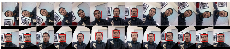
Fig. 6. Images captured by the front-facing camera assuming varying phone tilted angles from -90 \sim 90 degrees, separated by an angle of 15 degrees. The red boxes indicate the detection results. The first row is detected by the standard Adaboost face detector. The second row is detected by Visage’s detector.
