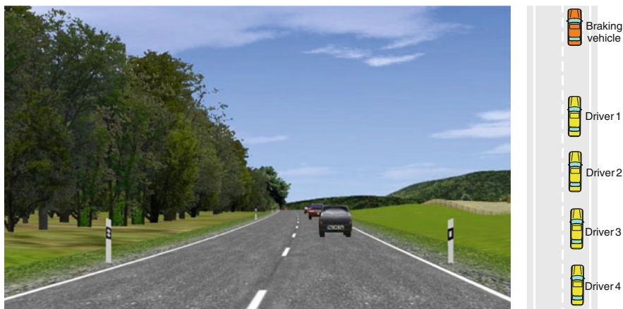
Fig. 11 Screenshots from the study ‘Braking vehicle’ with the rural road where the driving takes place ( left ) and illustration of the vehicles taking part in the scenario ( right )
