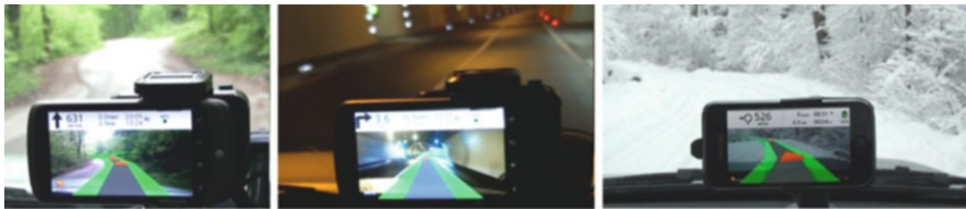
Fig. 9 The “Wikitude Drive” application overlays video captured through the camera with driving instructions and virtual road painting
