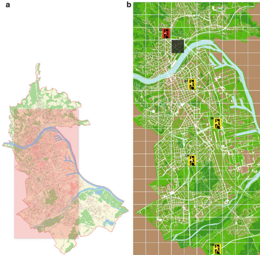
Fig. 7 (a) Original raster map of a city. Our agent-based model is simulated for the highlighted area. (b) The simulated city map, showing the 200 sectors as squares . Each sector was simulated by one processor. For the city-scale evacuation simulations, the exits (PoAs) are highlighted in yellow and red
