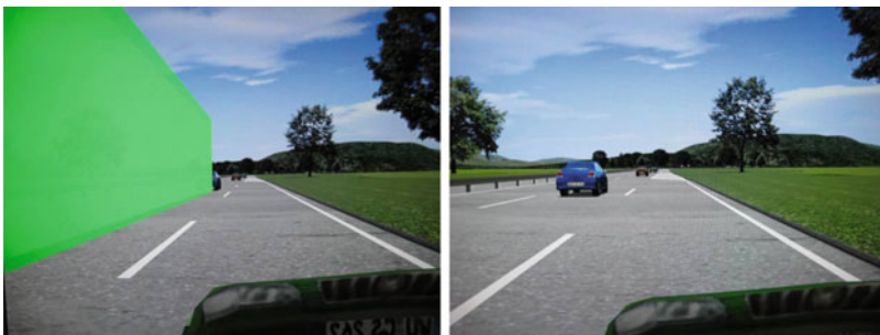
Fig. 17 Scenario of the study ‘Merging assistant’ with activated merging assistant ( left ) and without any assistance ( right )
