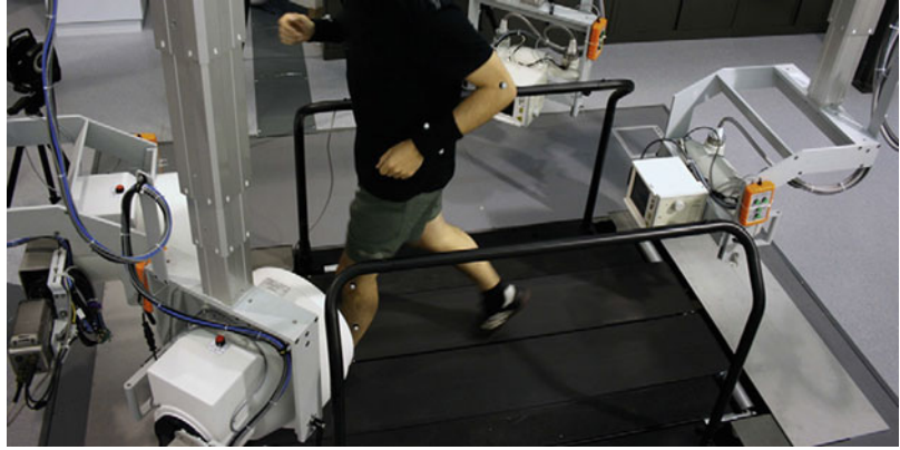
Fig. 6 A treadmill run test is shown with simultaneous biplane fluoroscopy of the knee (dynamic stereo radiography, DSX) (From Ahlden et al. (2012); needs permission from Springer Science and Business Media)
