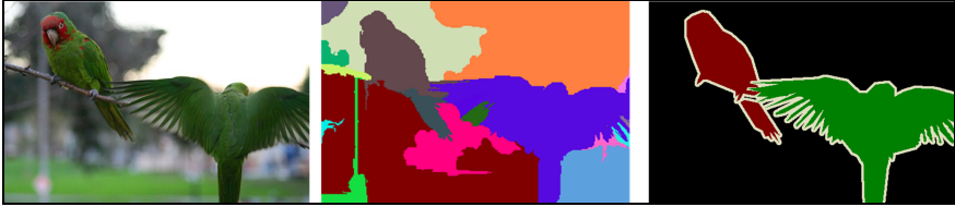
Fig. 4. Segmentation output: The input image (left) is transformed into a set of image regions (middle) or to segmented objects with black background and white boarder pixels (right)
