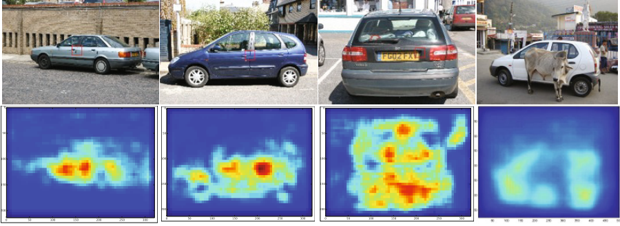
Fig. 5. The heat-maps shown in this figure are produced by mapping the scores of all the individual features on a plane. These show how the models locally learn the structures of the object.
