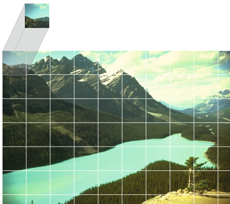
Fig. 3. Example demonstrating the application of near set theory to images, namely the image is partitioned into subimages where each subimage is considered a perceptual object, and object descriptions are the results of image processing techniques on the subimage
