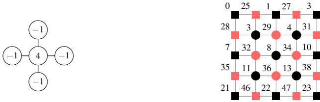
(a) Five-point stencil of the Poisson problem (3) discretized by finite differences on an equidistant grid. (b) Example of a red-black ordering. The rectangles note the border values given by the boundary condition.
