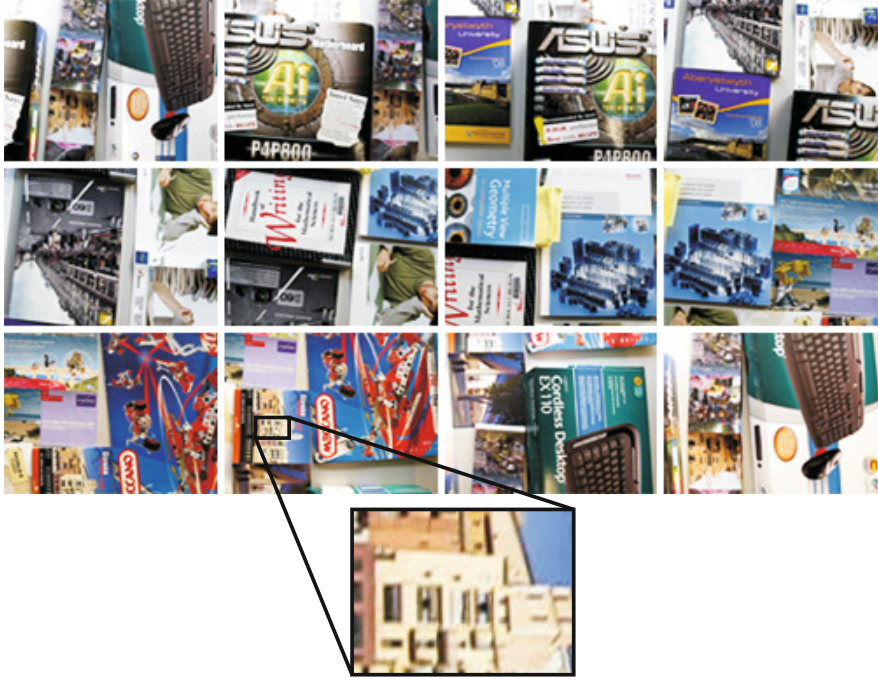
Fig. 4.7 Laboratory Experiment – Input image sequence. Sample images from the input sequence. The first and the last images have a partial overlap. The blow-up shows the motion blur and defocusing.
