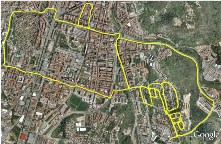
Fig. 4.15 Mixed Environment Experiment – Car trajectory during data acquisition. The 18.5 km trajectory (overlayed in yellow, as recorded by the DGPS system) was chosen to include multiple loop-closures. The starting point can be seen at the lower right corner.
