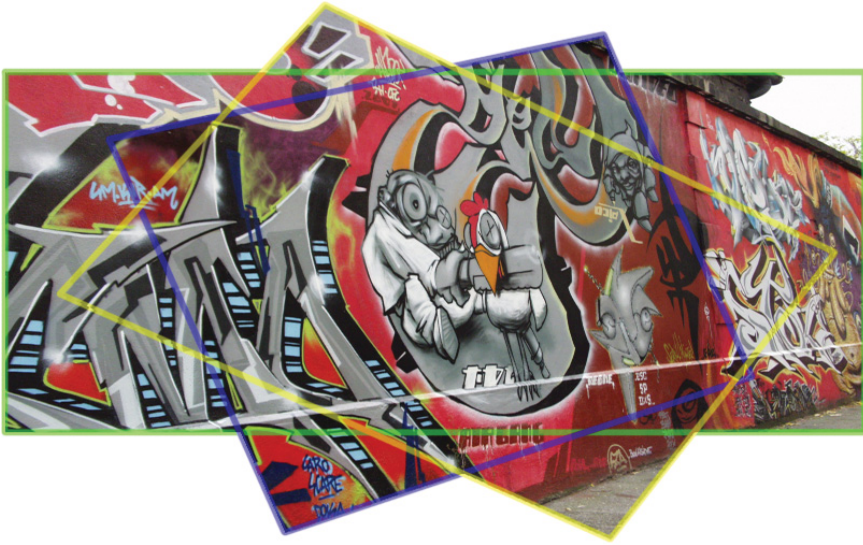
Fig. 2.7 Example of mosaicing. Mosaic of a planar scene. Colored rectangles outline of the contributing images. Green corresponds to the first (reference) frame, yellow and blue to the second and third images respectively. The mosaic was generated using the projective homography model.
