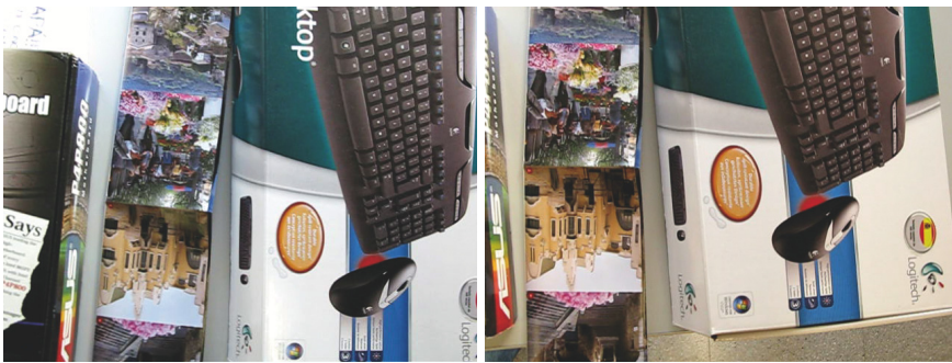
Fig. 4.13 Laboratory Experiment – Loop detection. The first (left) and last (right) images of the sequence correspond to the same region of the scene, determining a loop closure.
