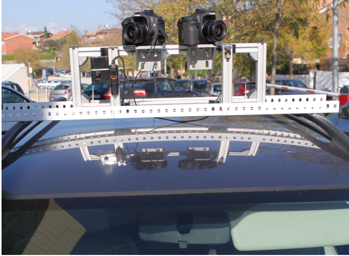
Fig. 4.14 Mixed Environment Experiment – Image acquisition setup. The dual-camera setup was mounted on a car during data acquisition.
