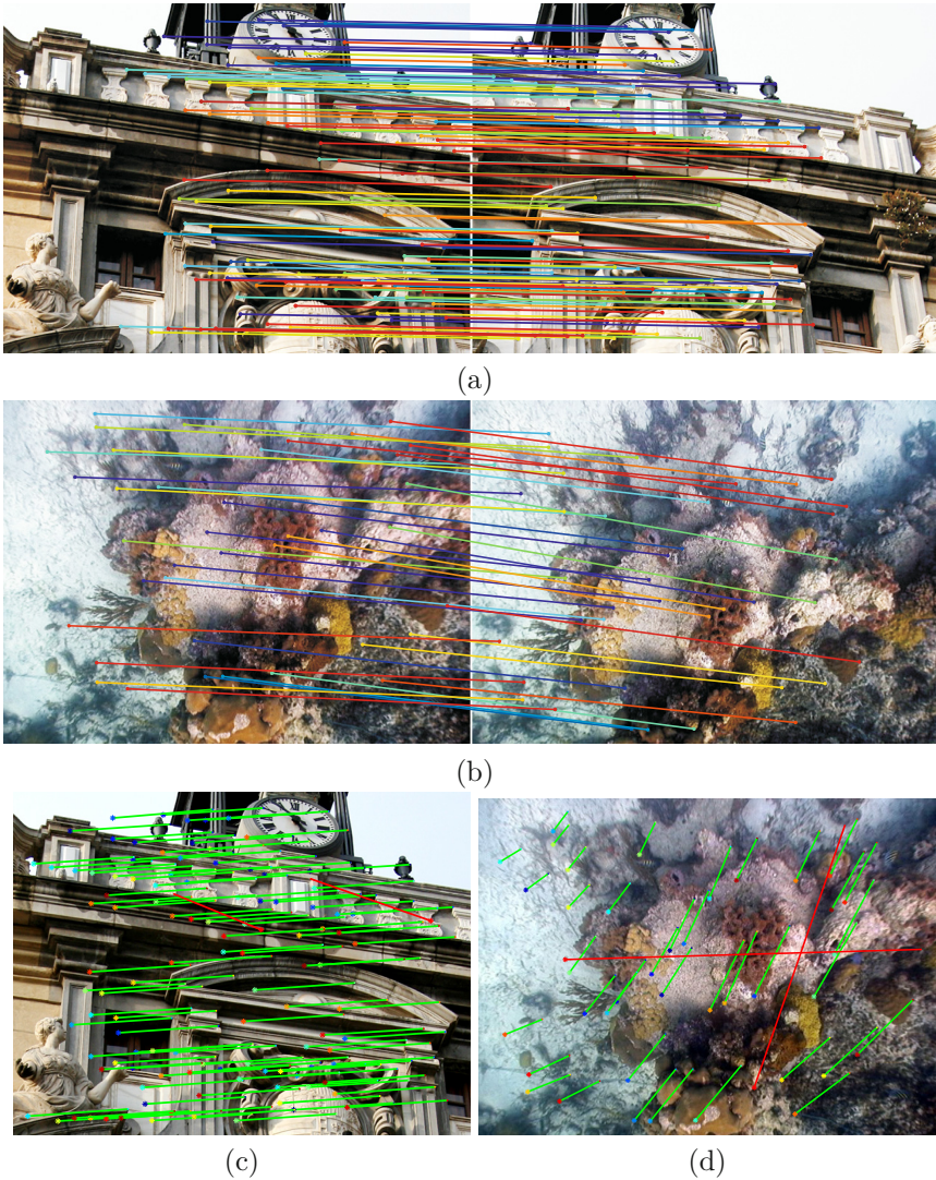
Fig. 2.6 Examples of feature matching. (a) and (b) illustrate matching between two images for an urban and an underwater scene. (c) and (d) show the disparity of the features. Red lines denote mismatched features (outliers).
