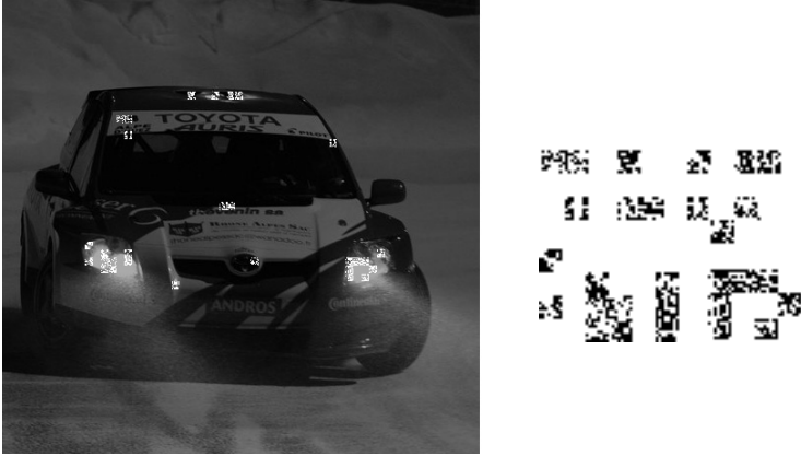
Fig. 1. Left: cover image '101.pgm' from BOSSbase compressed with quality factor 80. Right: close up of the recompression artifacts (grouped into a smaller region) with the same quality factor. The image contrast was decreased to better show the artifacts.
