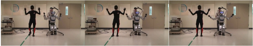
Fig. 3 Teleoperation with mixed given motion: The upper body of the humanoid has a joint motion comes from the motion capture suit and the lower body of the humanoid has a Cartesian motion which represents the foot print. Two different input motions are combined with the MECoM Jacobian. The lower body of the humanoid has delayed by about two steps because of the detection procedure of the human walking motion.
