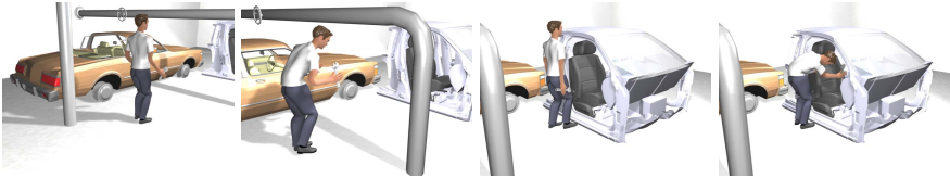
Fig. 4 Walking & Bending: The human model walks towards the car, avoiding some obstacles. It bends and stretches to put the tool inside the car
