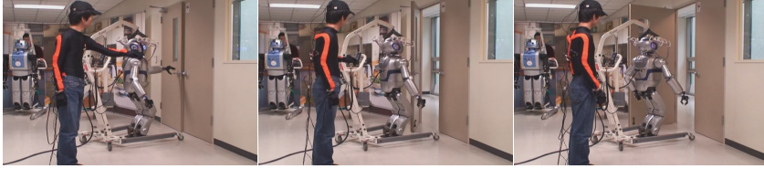
Fig. 4 Teleoperation with force control: In order to open a door, we embedded a compliance control algorithm into the upper body motion. By doing this, the embedded motion can follow the captured motion and can interact with an object in the environment simultaneously.
