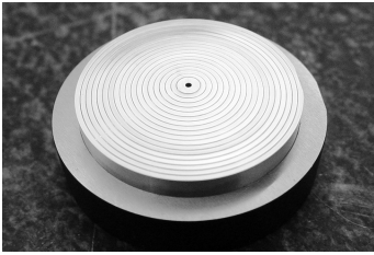
Fig. 2 Novel multi step-height artifact for the calibration of high frequency errors
