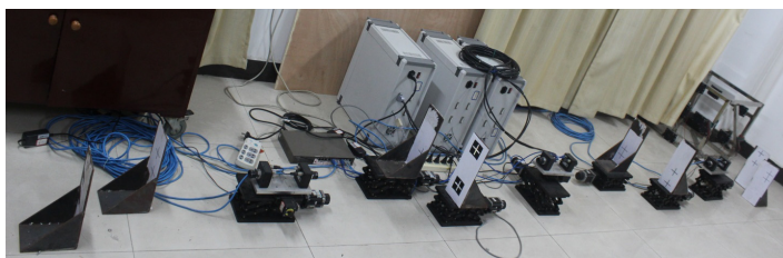
Fig. 4 Layout of the experimental subsidence measurement system
