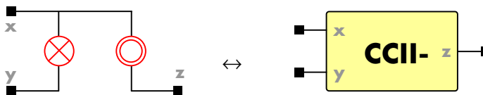
Fig. 14.21 The CCII- nullor equivalency
