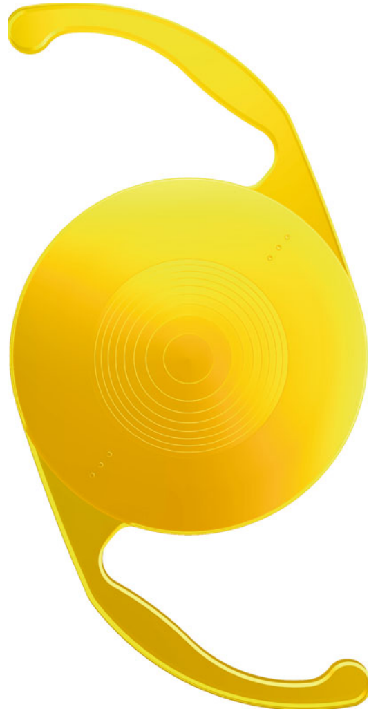
Fig. 7.2 Toric, aspheric, diffractive-refractive, circular, blue-light-filtering multifocal IOL (ReSTOR Toric, Alcon). The diffractive central zone allows for good near and distance visual acuity with small pupils; the peripheral zone is optimized for distance visual acuity with large pupils, for example, in night driving. The three dots indicate the cylinder axis
