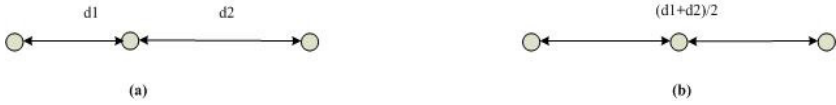
Fig. 1. Topology of a two-hop link. (a) Relay node deviating from the route midpoint, (b) relay node at the route midpoint.
