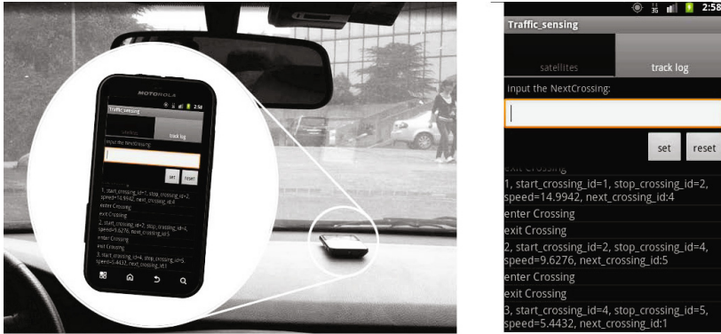
Fig. 5. The placement of the smartphone in a vehicle and the userface of smartphone
