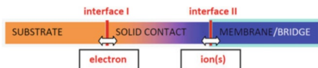
Fig. 10.1 Solid contact as ion-to-electron transducer. Ion-to-electron coupling scheme
