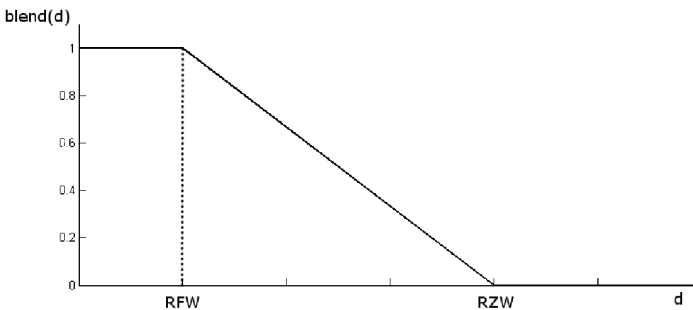
Fig. 2 Blending function for grid node deformation computation, including the parameter radius full weight (RFW) and radius zero weight (RZW)
