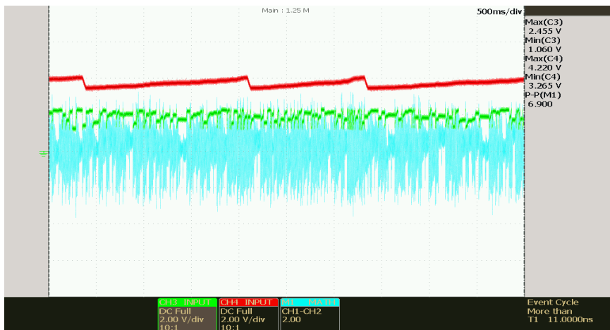
Fig. 6. The SEPIC output, depicted by the red-colored waveform
