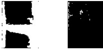
Fig. 4. Image of black sugarcane nodes and stem processed by binarization
