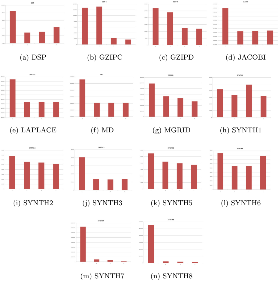
Fig. 9. Cycle counts for all applications for an unoptimized one buffer, an optimized one buffer, optimized two buffers and optimized four buffer versions
