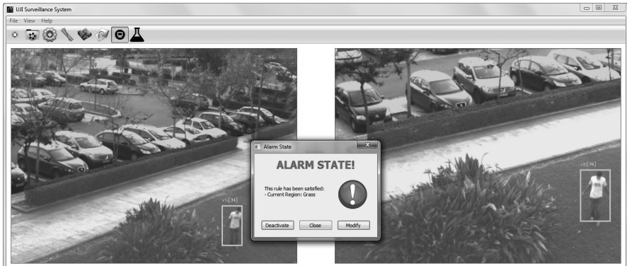
Fig. 3 An alarm rule is satisfied when a subject enters to the grass area
