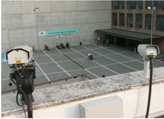
Fig. 11 The scene is surveyed from atop the CVC building using one fixed (right one in the image) and one active camera (left)
