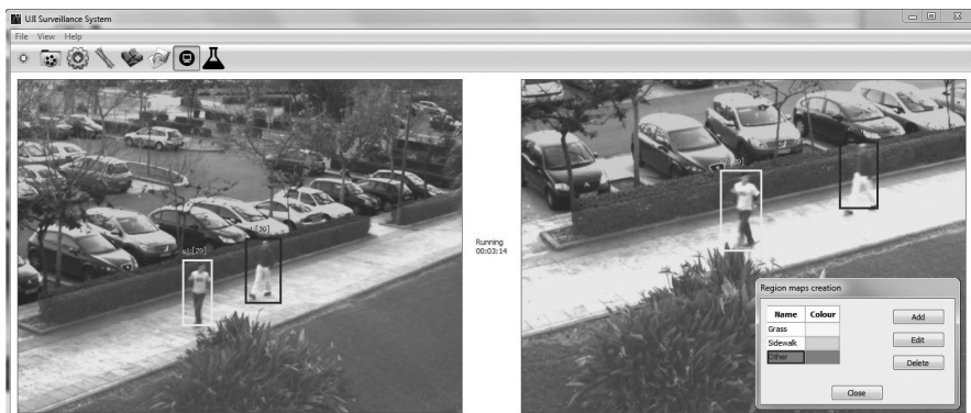
Fig. 2 An example of two-camera object tracking. The two silhouettes of a same subject share a common colour in their bounding box edges and an identical numeric label.
