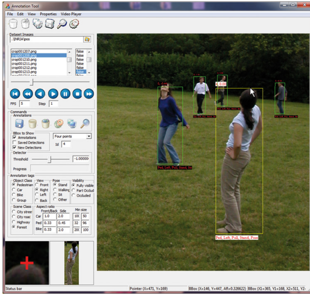
Fig. 6 Labelling tool. For each displayed image, the human oracle (Fig. 2) performs as follows: (1) if there are not humans, it marks the image as human-free ; (2) if there are humans, some of them have been detected by the previous classifier (green bounding box), but others may not (not framed). The undetected humans must be manually framed by the human oracle (yellow bounding box).
