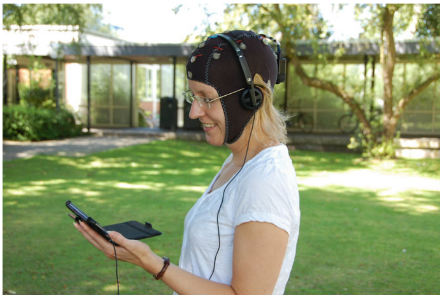
Fig. 19.5 A new wireless, fully head-mounted EEG system developed at Oldenburg University, Germany (Debener et al. 2012). The system allows for truly mobile EEG recordings, data can be recorded with a smartphone. Note that the cable is used for sound stimulus delivery, not for signal acquisition
