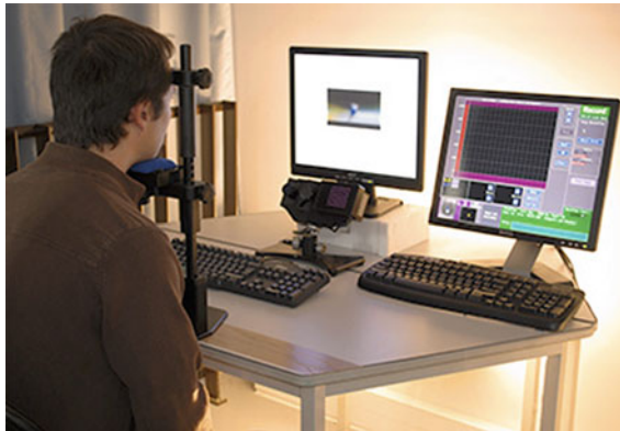
Fig. 25.4 Setup of a remote eye-tracker. The picture shows as an example of a laboratory setup the EyeLink 1000 eye-tracker (SR Research Ltd.). The infrared light source and camera are placed remotely, beneath the monitor that displays the stimulus for the participant. A chinrest is used to minimise head movements. Picture used with permission from SR Research Ltd.
