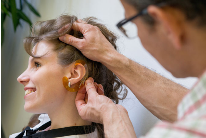
Fig. 19.6 The cEEGGrid, a flex-printed array of miniature EEG electrodes placed with an adhesive around the ear. This approach enables, unobtrusive, near invisible EEG acquisition (Debener et al. 2015)
