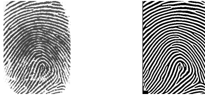
Fig. 2. (a) Typical Fingerprint image and (b) Enhanced image
