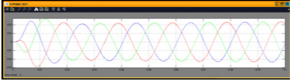
Fig. 6. Graphical results of Three-phase output of the Three wind plants with STATCOM
