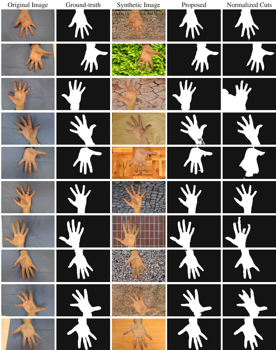
Fig. 4. A comparative study of results provided by segmentation algorithm in comparison to ground-truth. First column gathers examples from first database, together with their segmentation on second column, considered as ground truth. Third column presents synthetic images based on first column images, providing on the fourth column the final segmentation result. Last column presents the segmentation result provided by Normalized Cuts [16], respectively.
