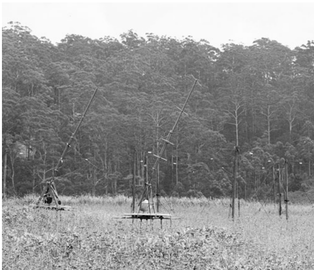
Fig. 9.2 The two Yagis used by Payne-Scott for solar work at the frequencies of 60 and 65 MHz at Hornsby Valley in 1948. The additional Yagi at 85 MHz is not shown; this consisted of a pair of crossed Yagis for reception of circular polarization. From 11 February 1948 (CSIRO Radio Astronomy Image Archive B1266-2)
