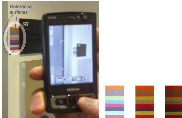
Fig. 1. Left: An example of application of the proposed technique. A marker with 9 color patches (two of which are used for reference) is taken by a cell phone camera. Each color patch contains 7 bits of information. Right: crop-outs from images of the same marker under different illuminants exemplify the dramatic color variations undergone by the patches.
