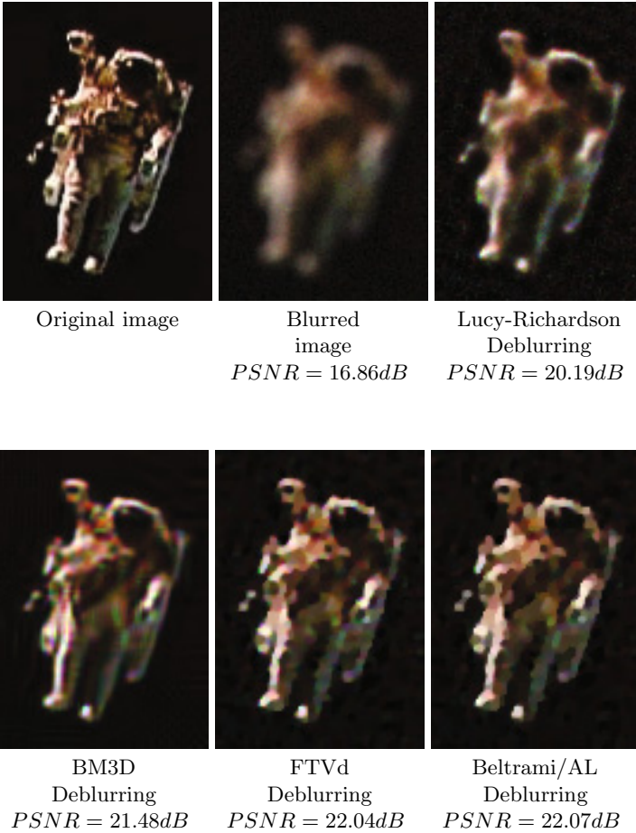
Fig. 4. Deblurring results with a disc blur filter of radius 5 and an Gaussian noise of \sigma = 5 . Left to right, top to bottom: (a) The original image. (b) The blurred image. (c) Deblurring using the Lucy-Richardson algorithm (d) BM3D-based deblurring. (e) Deblurring using the FTVd method. (f) Deblurring using the Beltrami / augmented Lagrangian algorithm.
