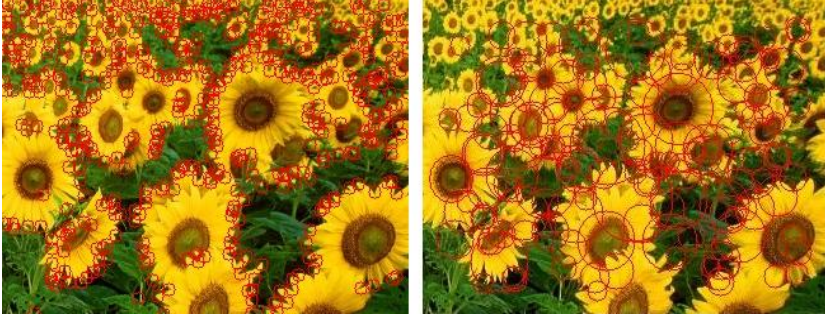
Fig. 1. Left: Interest points detected by Harris-Laplace. Right: Interest points detected by SURF. The red circles represent the detected features.
