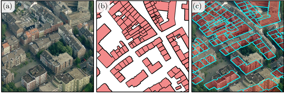
Fig. 1. Problem statement: Given a set of oblique aerial images (a) and a cadastral map (b), we compute the registration of the images with the map as shown in (c). Besides rough initial registrations, no further information is required. In particular, the cadastral map does not contain terrain elevation or building height information.
