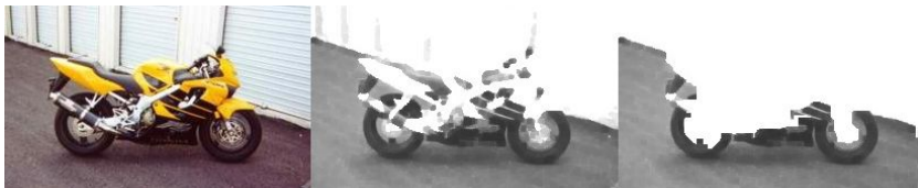
Fig. 5. A failure case: from left to right, the original image, the bright channel, and the refined bright channel. The uniformly dark road surface is identified as a shadow.
